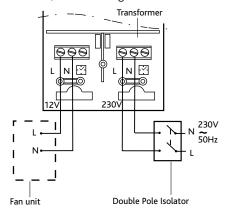
**SLIMAIRE 100XPC-12, 12V** with remote switch. (Pull-cord switch must be OFF before removing cord).
